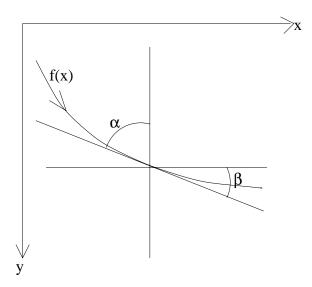
We consider the vertical plane P, containing the given points, A and B, and assume that A is higher than B. Then we introduce the rectangular coordinates in this plane, with the origin at A, horizontal x axis, and the y axis pointing down. Let y = f(x) be the function whose graph is the curve of minimal time from A to B.
