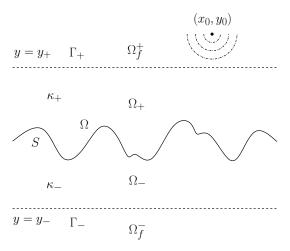
Figure 1: Problem geometry. A wave from the point source at  $(x_0, y_0)$  is incident on the scattering surface S from the top. The spaces  $\Omega_f^+$  (above S) and  $\Omega_f^-$  (below S) are filled with materials whose wavenumbers are constants  $\kappa_+$  and  $\kappa_-$ , respectively.
