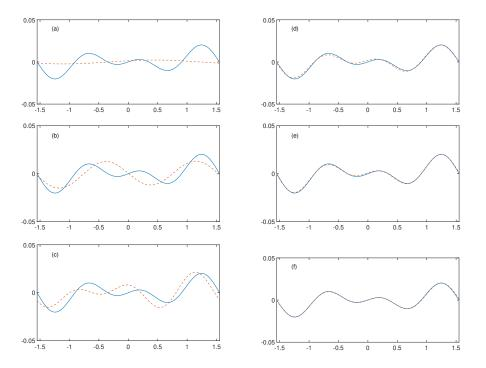
FIGURE 2. Example 1: the reconstructed surface (dashed line) is plotted against the exact surface (solid line). (a)  $\rho_1 = 1$ ; (b)  $\rho_1 = 2$ ; (c)  $\rho_1 = 4$ ; (d) 1 step of nonlinear correction when  $\rho_1 = 4$ ; (e) 2 steps of nonlinear correction when  $\rho_1 = 4$ ; (f) 3 steps of nonlinear correction when  $\rho_1 = 4$ .
