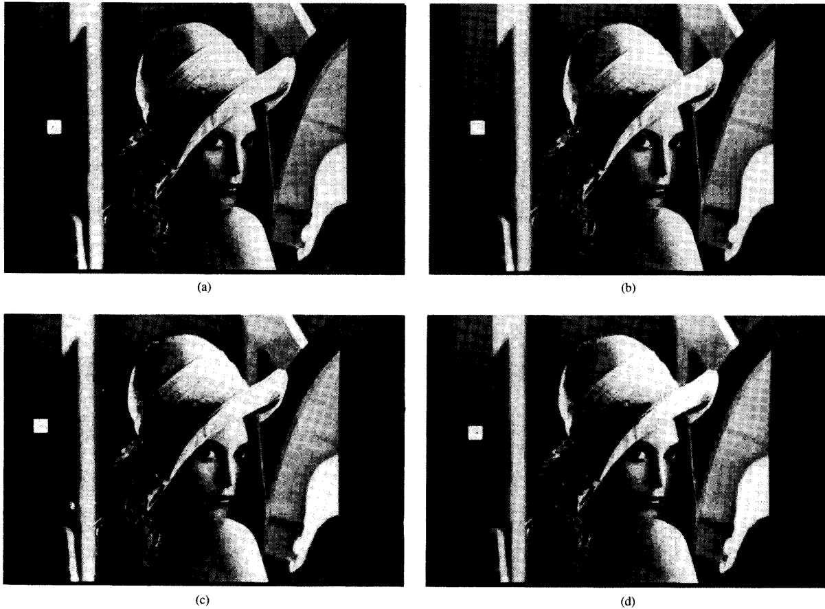
Fig. 3. Lenna, compressed using the L^1(I) quantization strategy: (a) original; (b) compressed with q = 128 (20 236 coefficients, 14 604 bytes); (c) compressed with q = 256 (12 068 coefficients, 8925 bytes); (d) compressed with q = 512 (7001 coefficients, 5404 bytes).
