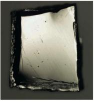
Electrons move along the surface of, but not through, topological insulators such as bismuth selenide.
