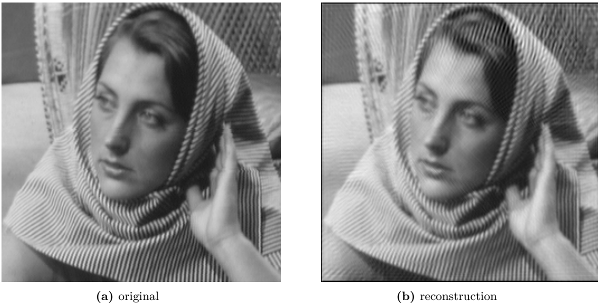
Figure 9. The Barbara image on a 250 \times 250 grid, reconstructed with iradon from its Radon transform computed with radon . The one degree angular resolution creates non-local aliasing artifacts.
