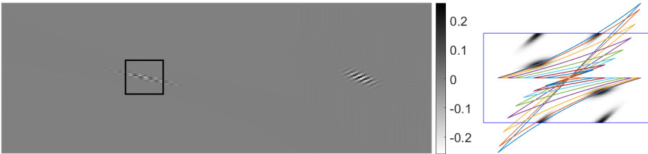
Fig. 13: Left: vertically subsampled data, the boxed singularity on the left is aliased. Right: modulus of Fourier transform of I_0 f with bowties superimposed. The surrounding blue box is the frequency range allowed by the sampling.
