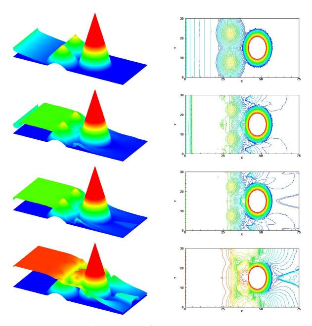
Figure 4.6: The water surface level in the flooding problem on a channel with three mounds at different times  $t=8,\,30,\,300$  and 540 (from top to bottom). Left: 3D view, color spanning between 0 and 1.2; Right: the 2D contours with 30 uniformly spaced contour lines between 0 and 1.2.
