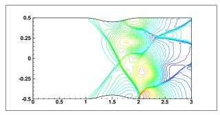
Figure 4.11: The contours of the water surface level of the converging-diverging channels problem in Section 4.7 with the parameters d=0.9 and B=2. Results are based on the triangulation with mesh sizes  $\tau_K=0.025$  (left) and 6.25E-03 (right), respectively.
