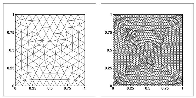
Figure 4.1: The computational domain and unstructured triangular meshes of the accuracy test problem in Section 4.2. Left: with mesh size  $\tau_K = 0.1$ ; Right: with mesh size  $\tau_K = 0.025$ .
