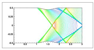
Figure 4.8: The contours of the water surface level of the converging-diverging channels problem in Section 4.7 with the parameters d = 0.9 and B = 0. Results are based on the triangulation with mesh sizes  $\tau_K = 0.025$  (left) and 6.25E - 03 (right), respectively.
