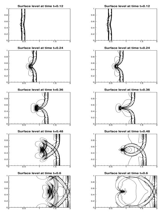
Figure 4.2: The contours of the surface level h+b for the problem in Section 4.3. 40 uniformly spaced contour lines. From top to bottom: at time t=0.12 from 0.999993 to 1.00007; at time t=0.24 from 0.9999 to 1.0001; at time t=0.36 from 0.9998 to 1.0002; at time t=0.48 from 0.99985 to 1.00005; and at time t=0.6 from 0.9999 to 1.0001. Left: results with the bottom (4.2). Right: results with the bottom (4.4).
