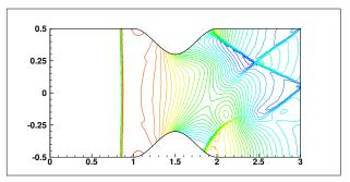
Figure 4.10: The contours of the water surface level of the converging-diverging channels problem in Section 4.7 with the parameters d=0.6 and B=1. Results are based on the triangulation with mesh sizes  $\tau_K=0.025$  (left) and 6.25E-03 (right), respectively.
