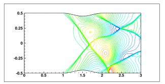
Figure 4.9: The contours of the water surface level of the converging-diverging channels problem in Section 4.7 with the parameters d = 0.9 and B = 1. Results are based on the triangulation with mesh sizes  $\tau_K = 0.025$  (left) and 6.25E - 03 (right), respectively.
