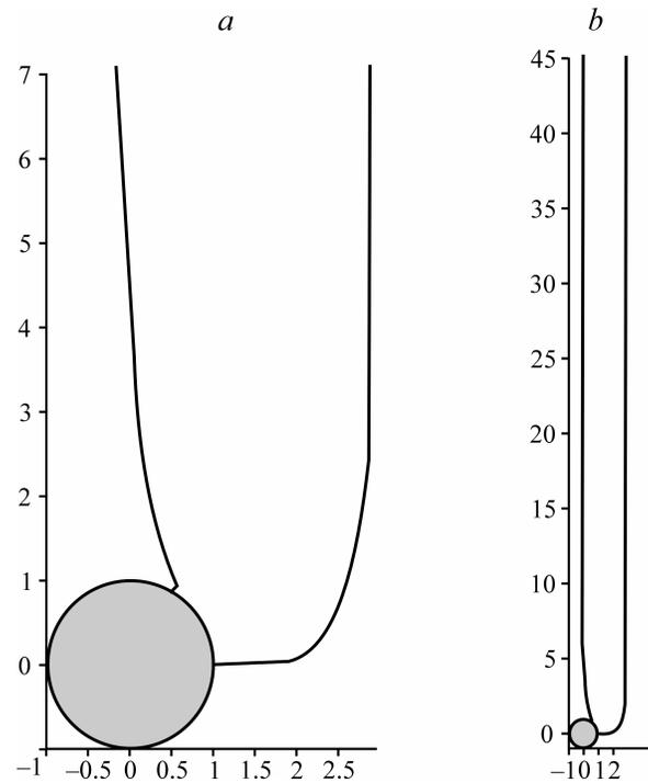
Fig. 4. Two phases of the hydraulic fracture propagation with initial fractures oriented at  $0^\circ$  and  $60^\circ$ :
