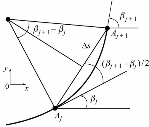
Fig. 2. Calculation scheme for the fracture trajectory
