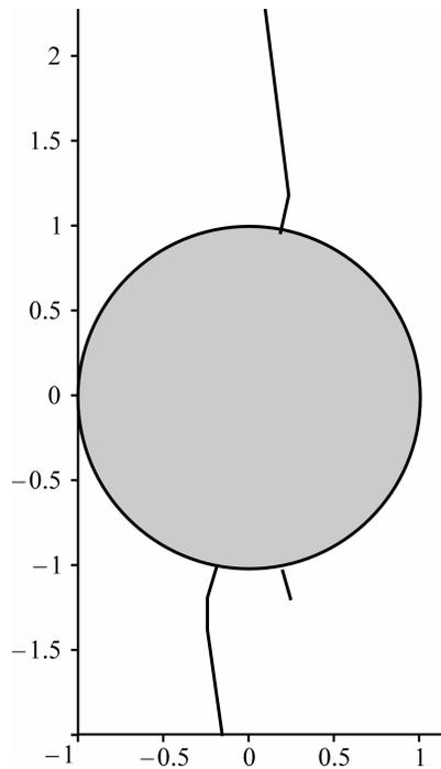
Fig. 5. Trajectories for three hydraulic fractures coming out of the same well, at the initial fracture angles of  $80^\circ$ ,  $258^\circ$  and  $284^\circ$
