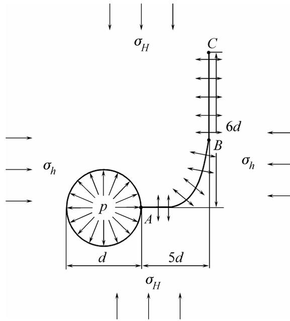
Fig. 3. Estimate for the role of digitizing the well contour and the “rear” portion of the hydraulic fracture
