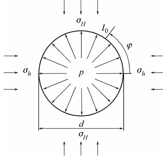
Fig. 1. Calculation scheme for modeling a hydraulic fracturing process: horizontal section of a well and an initial crack
