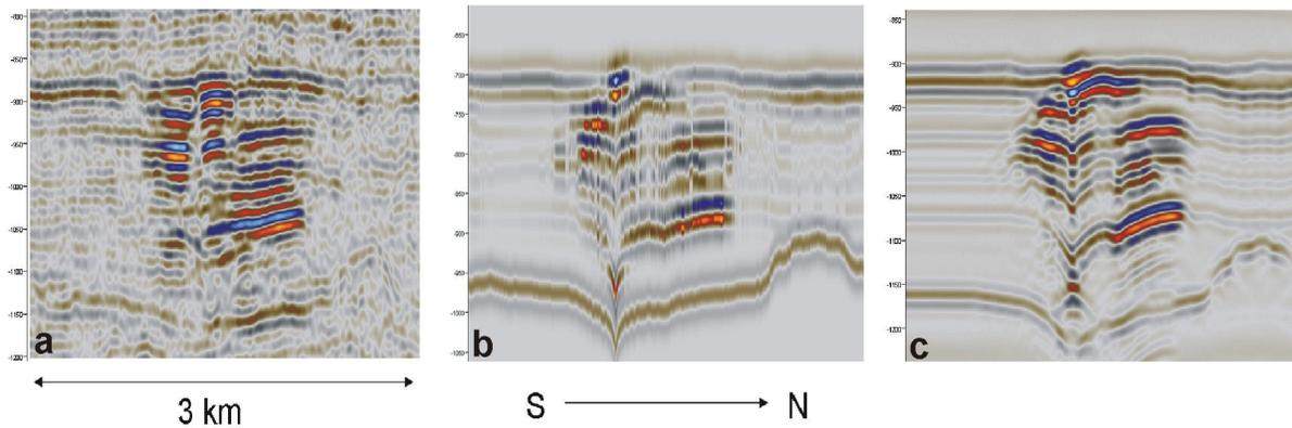
Figure 6 A comparison between a) the observed inline from the 1999 seismic survey; b) the corresponding synthetic line obtained by convolutional modeling and c) the corresponding synthetic line after 2D elastic modelling and processing
