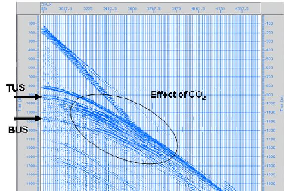
Figure 4 Synthetic shot gathers generated by elastic pre-stack modelling. Source and streamer are above the CO<sub>2</sub> plume which is imaged on mid-offset traces. Note enhanced reflectivity in the reservoir, but reduction of coherence in deeper reflections due to lateral velocity changes TUS = Top Utsira Sand; BUS = Base Utsira Sand.
