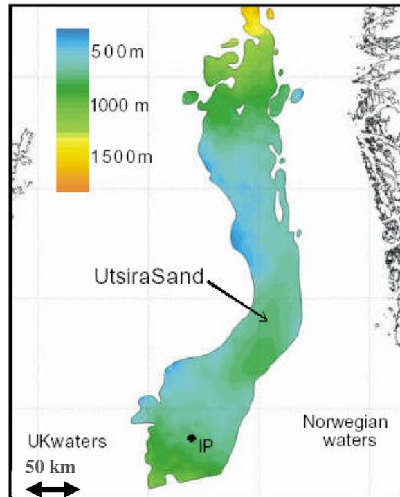
Figure 1: Depth map of the Utsira Sand with the CO<sub>2</sub> injection point (IP) indicated. Note that the area currently occupied by the CO<sub>2</sub> is less than 3 km<sup>2</sup>.
