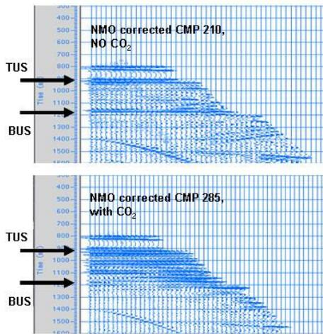
Figure 5: Comparison between a synthetic CMP gather without CO<sub>2</sub> (upper) and with CO<sub>2</sub> (lower) present.
