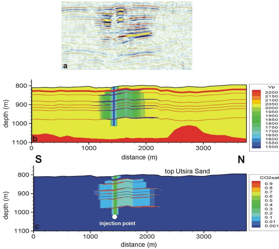
Figure 3 Detailed model of the Sleipner plume in 1999 derived from acoustic modelling. Seismic inline 3838 (top), modelled Vp (centre), modelled CO<sub>2</sub> saturation (bottom). Note the vertical column of velocity pushdown and reduced reflectivity interpreted as a vertical feeder chimney of higher saturation CO<sub>2</sub>.
