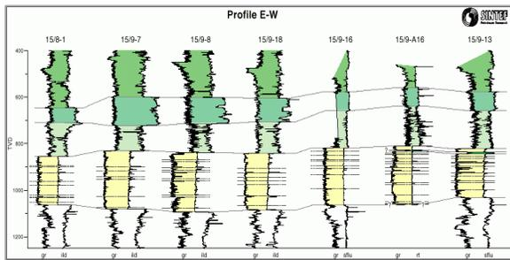
Figure 2: East-West correlation panel of the different well logs (gamma ray and resistivity logs) penetrating the mudstone-siltstone overburden (in green) and the Utsira Sand reservoir (in yellow). Note the uncorrelated thin shale layers appearing as peaks in the Utsira reservoir.
