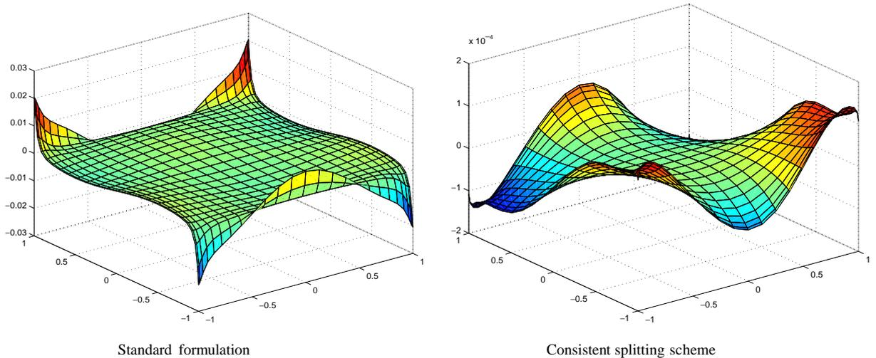
Fig. 4. Pressure error field at time  $t = 1$  in a square. Standard formulation vs. consistent splitting scheme.
