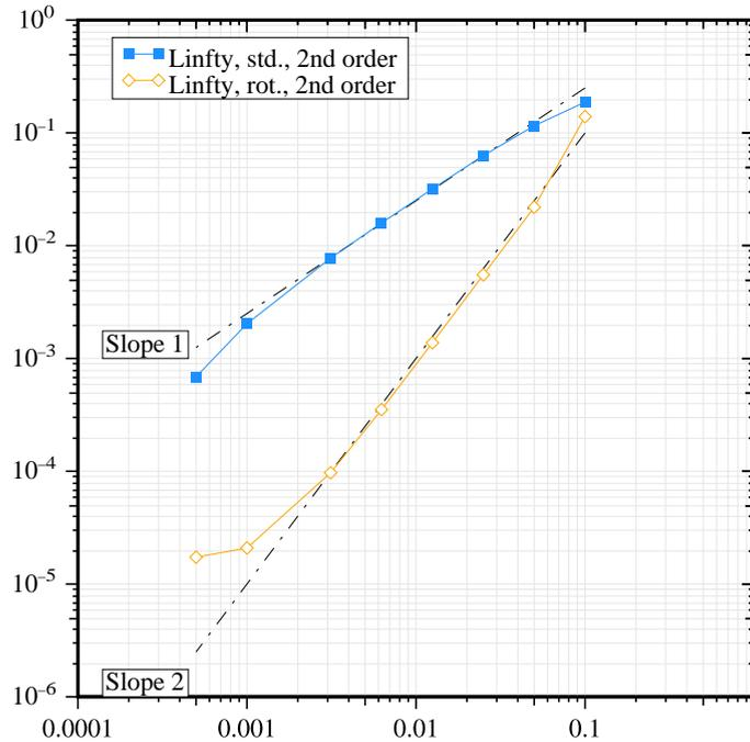
Fig. 2. Convergence tests with BDF2 and Finite elements. Error on the pressure in the  $L^\infty$ -norm at  $T = 1$ . Standard formulation vs. rotational formulation.
