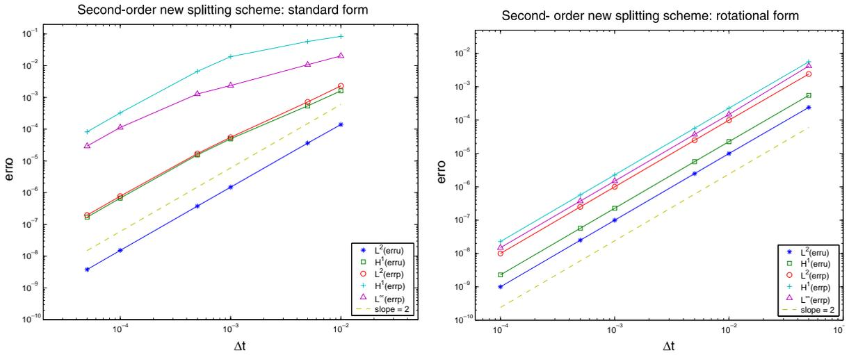
Fig. 3. Convergence rates with spectral approximation. \*: velocity,  $L^2$ -norm;  $\square$ : velocity,  $H^1$ -norm;  $\circ$ : pressure,  $L^2$ -norm;  $+$ : pressure,  $H^1$ -norm;  $\triangle$ : pressure,  $L^\infty$ -norm. Standard formulation vs. consistent splitting scheme.
