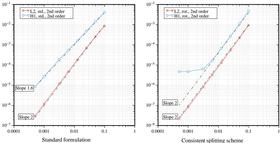
Fig. 1. Convergence tests with BDF2 and Finite elements. Error on the velocity in the  $L^2$ -norm and in the  $H^1$ -norm at  $T = 1$ . Standard formulation vs. consistent splitting scheme.
