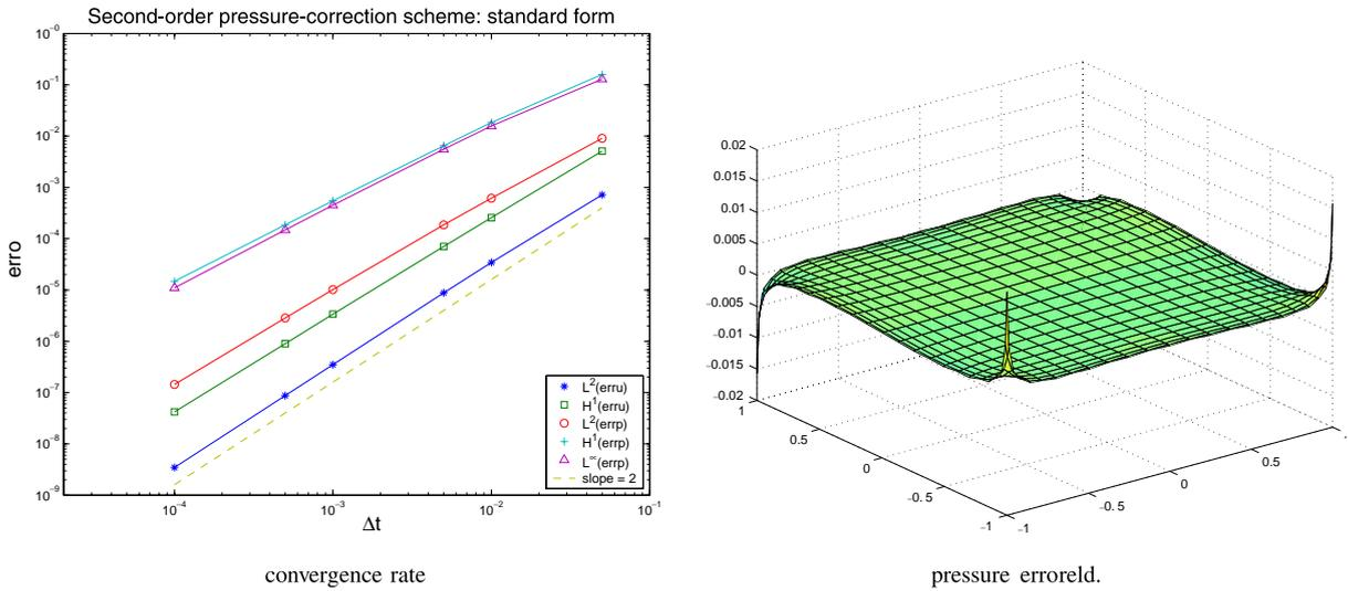
Fig. 5. Second-order rotational pressure-correction. \*: velocity,  $L^2$ -norm;  $\square$ : velocity,  $H^1$ -norm;  $\circ$ : pressure,  $L^2$ -norm;  $+$ : pressure,  $H^1$ -norm;  $\triangle$ : pressure,  $L^\infty$ -norm. Convergence rate vs. pressure error field.
