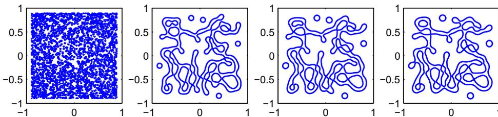
**Fig. 2.** The time evolution of the gradient-flow equation in PEM, implemented with scheme (5.8). The blue lines are interfaces drawn at four different time spots. It starts from the random initial condition. The Legendre–Galerkin method is used with  $129 \times 129$  Gaussian points. The terminal time is  $T = 12$ . The time step size is  $\delta t = 0.01, s_1 = s_2 = 2$  and  $\epsilon = 0.02$ .
