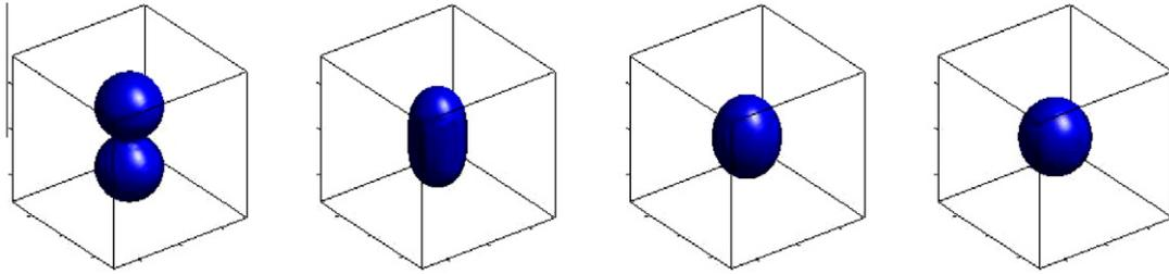
**Fig. 1.** The time evolution of the Cahn–Hilliard Eq. (5.2). The four plots are zero-isocontours of  $\phi$  at  $t = 0, \frac{T}{3}, \frac{2T}{3}, T$ , with  $T = 0.9, \delta t = 0.001, \epsilon = \gamma = 0.02, s = 1$ . The Legendre–Galerkin method is used with  $91 \times 91 \times 91$  Legendre–Gauss–Lobatto points.
