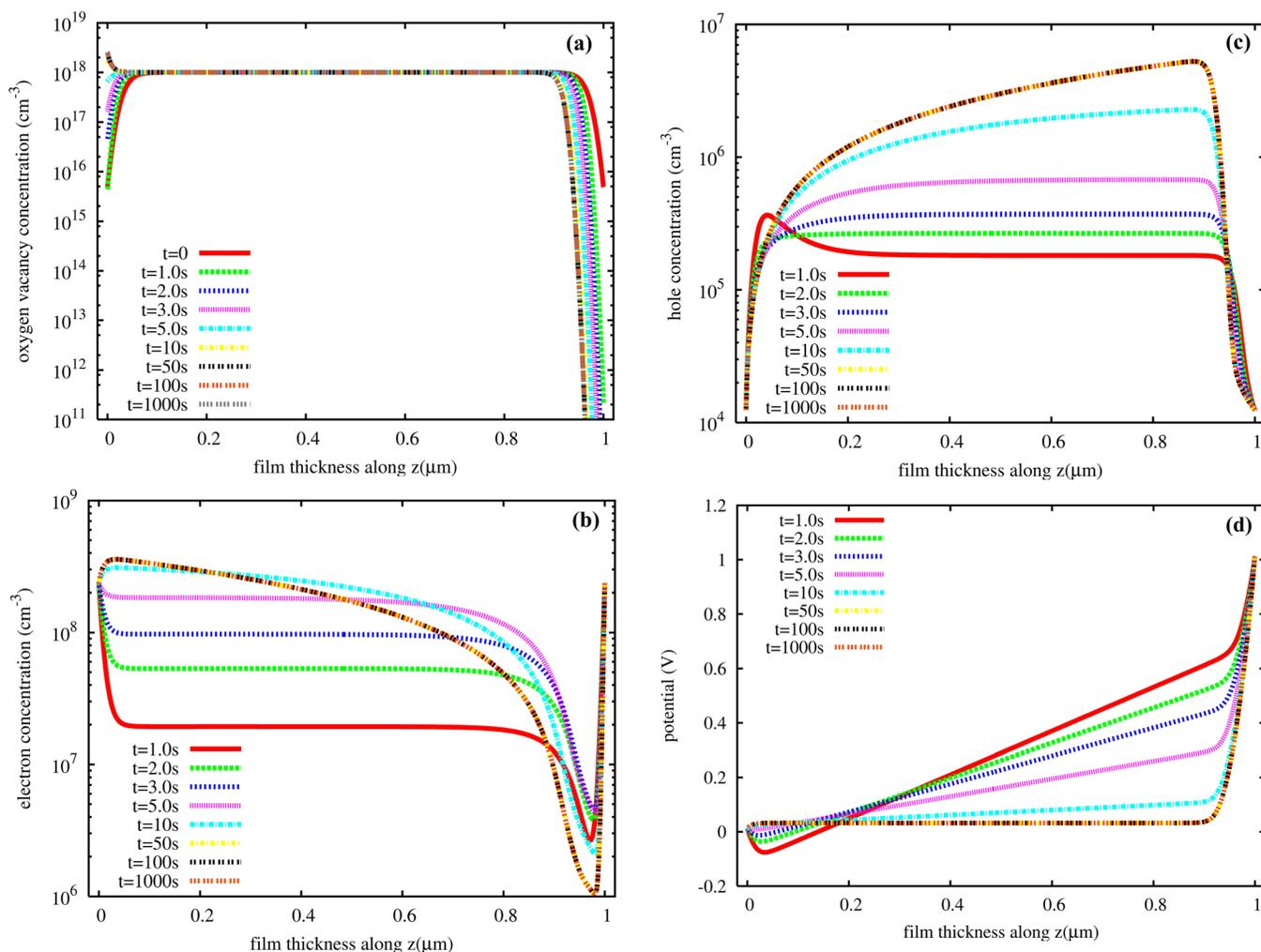
FIG. 4. Evolution of charged defects and electric potential profile to steady state for SrTiO<sub>3</sub> at  $T = 150^\circ\text{C}$  under a 1.0V external bias (a) oxygen vacancy; (b) electron; (c) hole, and (d) electric potential profile.
