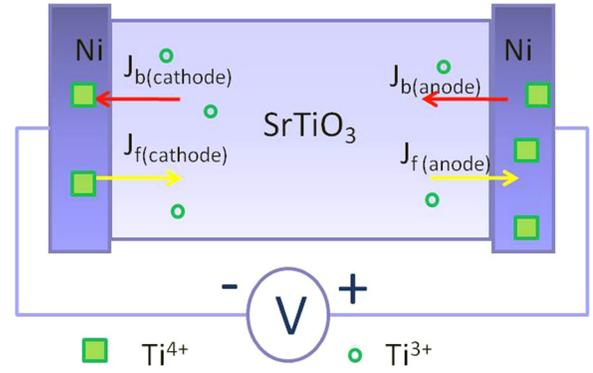
FIG. 2. Schematic plot of the Ni/SrTiO<sub>3</sub>/Ni sandwich structure and the small polaron hopping between Ti<sup>3+</sup> and Ti<sup>4+</sup> ( $Ti^{4+} + e^- = Ti^{3+}$ ).
