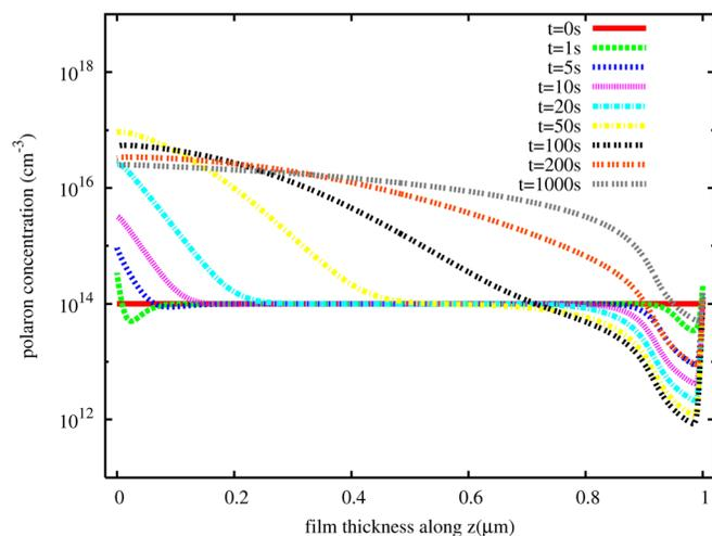
FIG. 6. Evolution of polaron under flux boundary condition in SrTiO<sub>3</sub> under 1.0 V dc bias.
