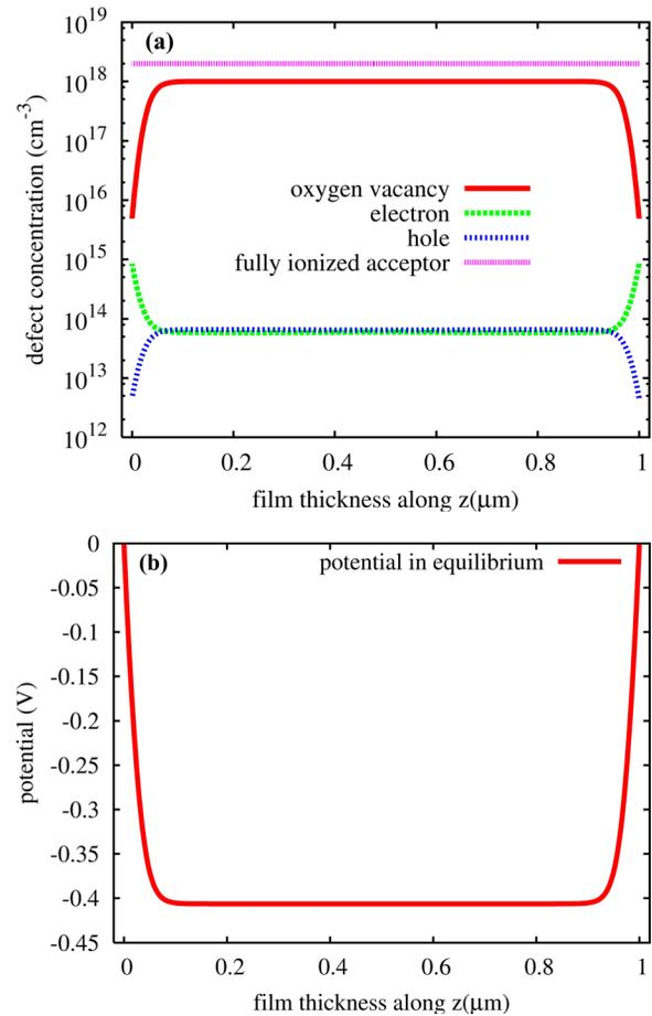
FIG. 3. The ionic/electronic charged defects and inner potential distribution in equilibrium SrTiO<sub>3</sub> single layer of 1 μm in thickness at  $T = 1000 \text{K}$  (with no external applied potential bias). (a) oxygen vacancy, electron, hole, and fully ionized acceptors; (b) inner potential profile.
