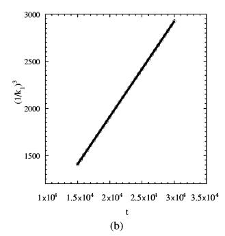
FIG. 6. The cubic of the average domain size vs time at the late stage of bulk-diffusion-controlled coarsening: (a) domain size characterized by  $R_g$ ; (b) domain size characterized by  $(1/k_1)$ .
