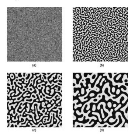
FIG. 1. Morphological patterns during spinodal decomposition and subsequent coarsening for bulk-diffusion-controlled dynamics: (a) t= 100, (b) t = 2000, (c) t = 10 000, (d) t= 30 000.
