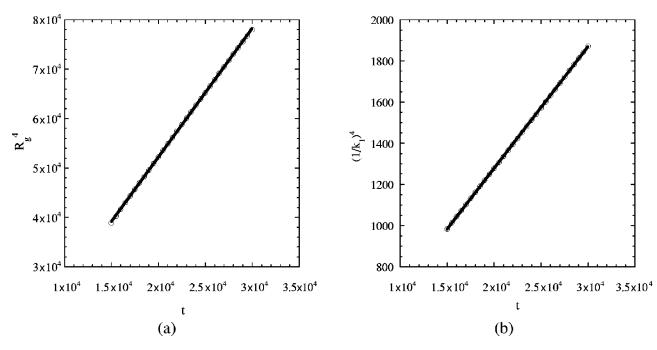
FIG. 7. The fourth power of the average domain size vs time at the late stage of interface-diffusion-controlled coarsening: (a) domain size characterized by  $R_g$ ; (b) domain size characterized by  $(1/k_1)$ .
