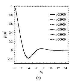
FIG. 5. Plot of the normalized pair correlation function g(r,t) vs  $rk_1$ : (a) for bulk-diffusion-controlled dynamics; (b) for interface-diffusion-controlled dynamics.
