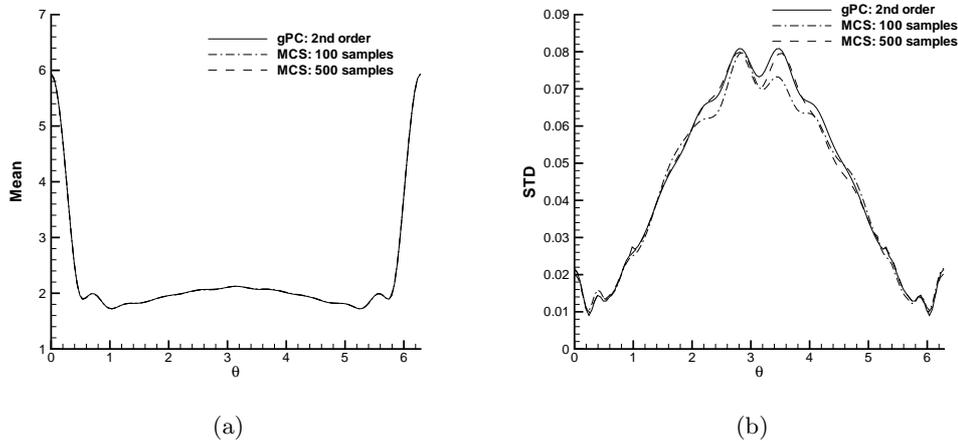
Figure 8: RCS profile of scattering over a rough gear-shaped obstacle. (a) Mean; (b) standard deviation.
