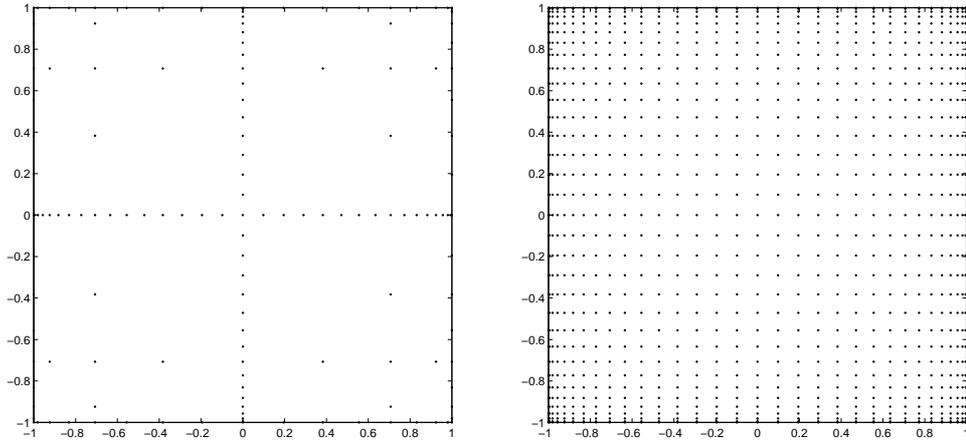
Figure 1: Two-dimensional ( $N = 2$ ) nodes based on the extrema of Chebyshev polynomials. Left: Sparse grid from Smolyak algorithm. Total number of points is 145. Right: Tensor product grid constructed from the same one-dimensional nodes. Total number of nodes is 1,089.
