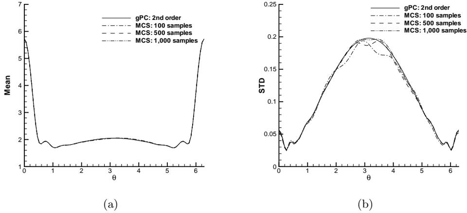
Figure 6: RCS profile of scattering over a rough cylinder. (a) Mean; (b) standard deviation.
