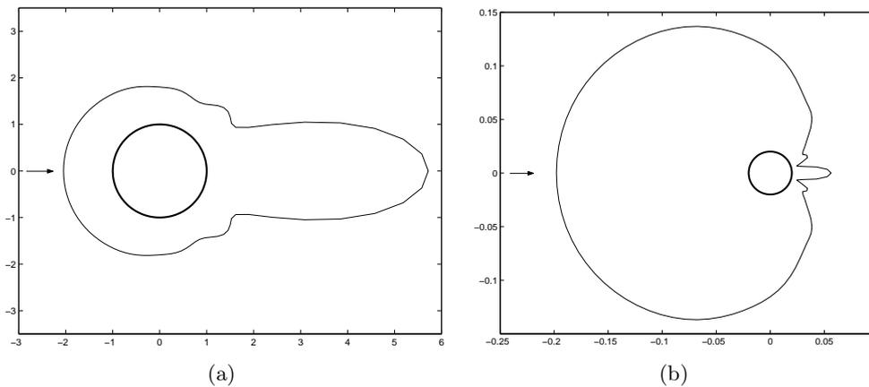
Figure 5: Acoustic scattering over cylinder with rough surface. The arrow indicates the direction of the incident plane wave. (a) The mean solution of RCS. The thick circle is the mean boundary of the scatterer; (b) Standard deviation of the RCS profile. Here the thick circle is only a reference of the location of the cylinder because of the scale difference.
