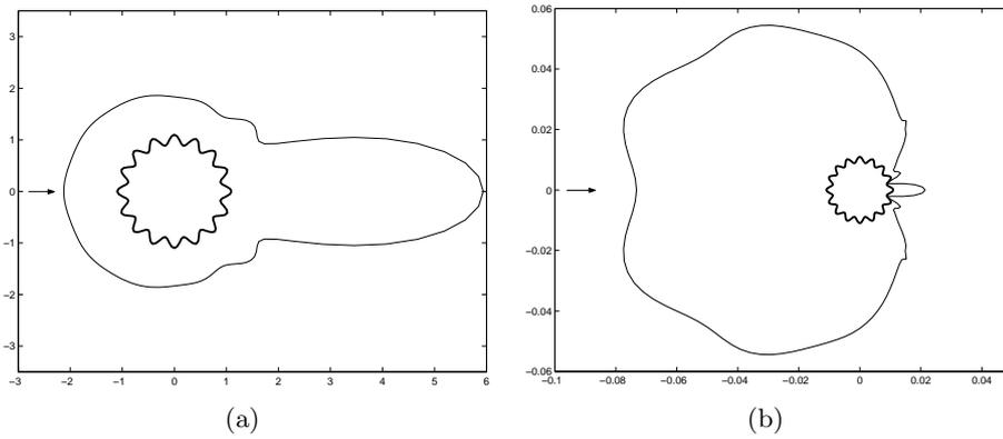
Figure 7: Acoustic scattering over cylinder with rough surface. The arrow indicates the direction of the incident plane wave. (a) The mean solution of RCS. The thick line is the mean boundary of the gear-shaped obstacle; (b) Standard deviation of the RCS profile. Here the thick line is only a reference of the location of the obstacle because of the scale difference.
