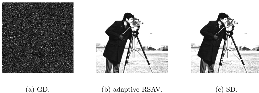
FIG. 6. Results after 20,000 iterations for a phase retrieval problem with z_* being a 256 \times 256 real image of camera man, m=6 Gaussian random masks and a random initial guess. The vanilla GD uses the nearly largest stable constant step-size \delta t = 0.5 .
