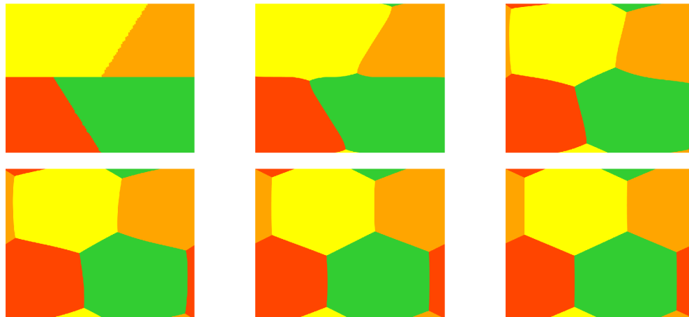
Figure 6: Example 4.5. A 4-subdomain partition: initial partition and subdomains at times T = 0, 0.05, 0.5, 1, 5, 10 computed by the second-order R-GSAV/LM scheme.
