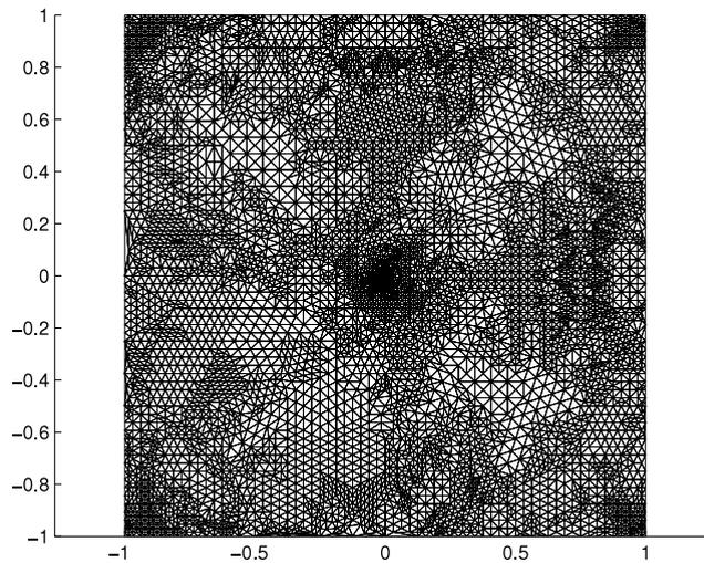
Fig. 5.4. Final adapted mesh,  $P_1 - RT_1$ , “Rough” solution.
