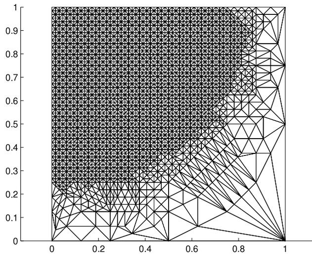
Fig. 5.2. Adapted mesh, smooth solution,  $P_1 - RT_1$ .
