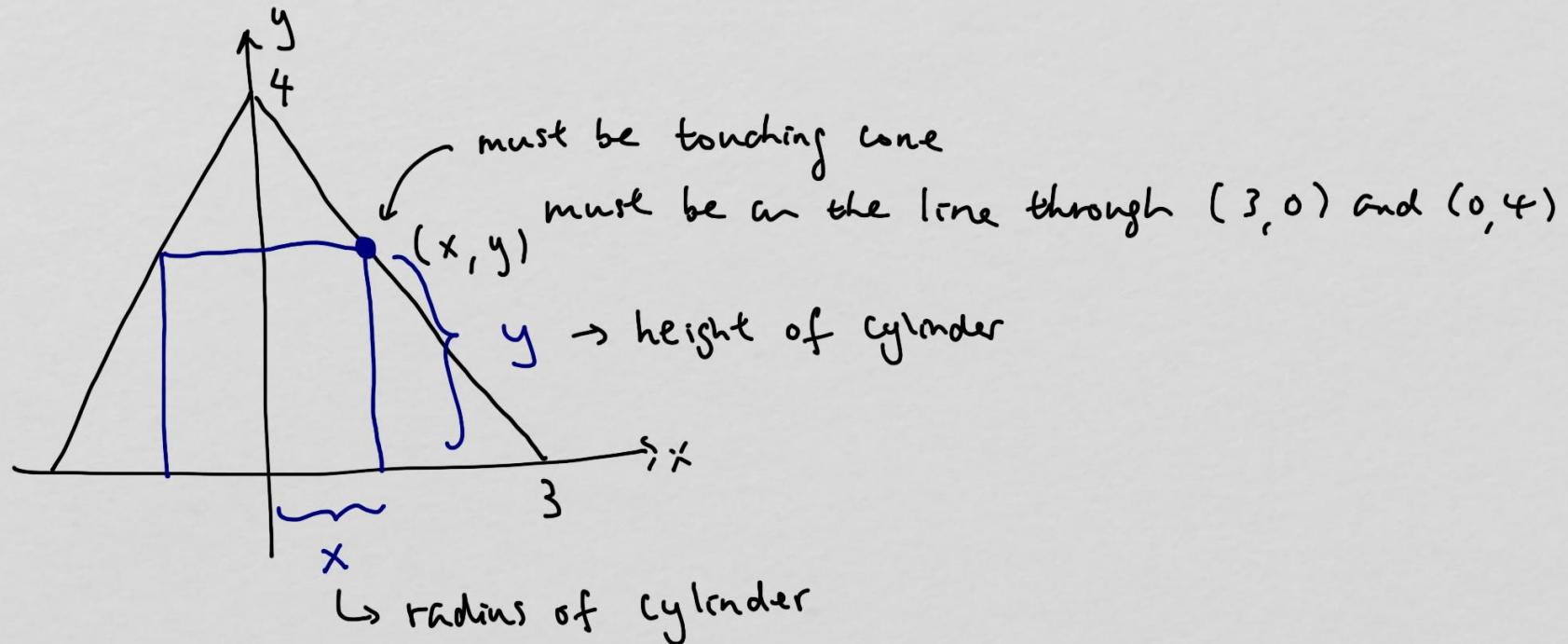
$$\text{volume of cylinder: } \pi x^2 y = V$$
