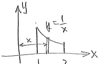
$$\begin{aligned}\bar{x} &= \frac{\bar{M}_y}{m} = \frac{\int_1^2 x \left( \frac{1}{x} - 0 \right) dx}{\int_1^2 \left( \frac{1}{x} - 0 \right) dx} \\ &= \frac{\int_1^2 1 dx}{\ln x \Big|_1^2} = \frac{x \Big|_1^2}{\ln 2} = \frac{2-1}{\ln 2} \\ &= \frac{1}{\ln 2}\end{aligned}$$
