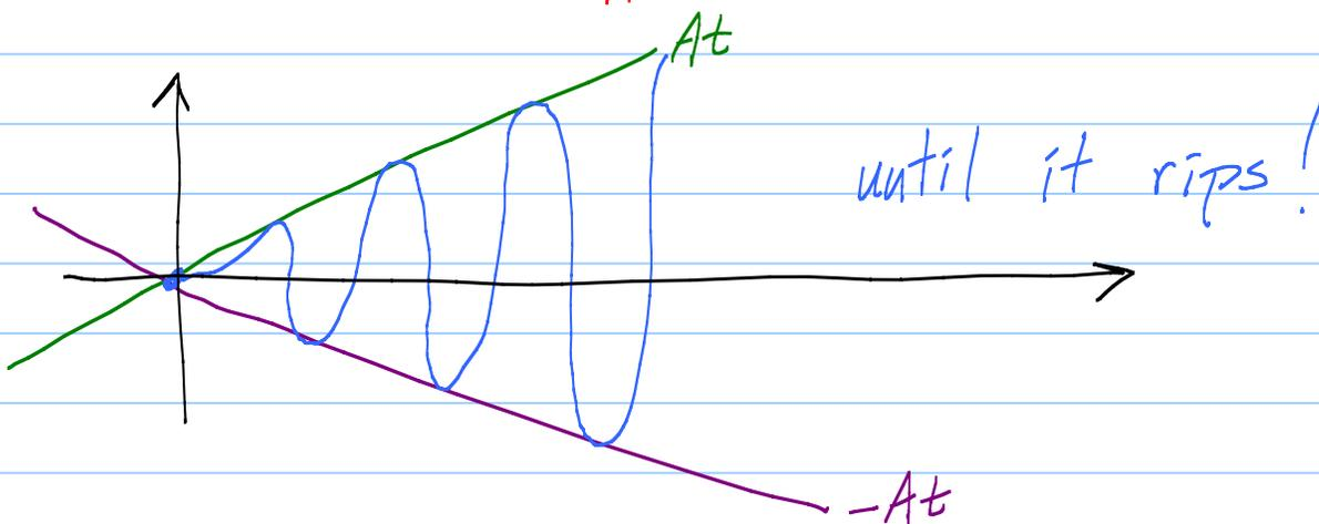
Damping  $m \ddot{y} + c \dot{y} + k y = F_0 \cos \omega t$
