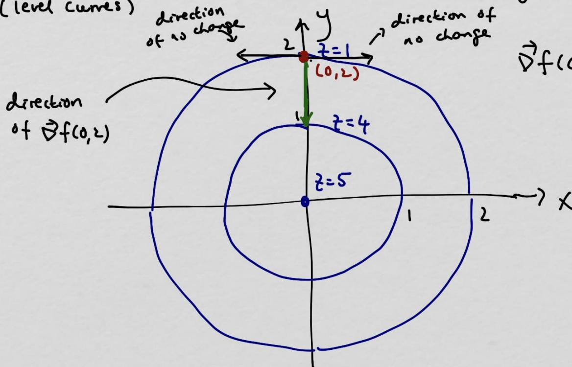
it looks like to get the maximum directional derivative, we want to go orthogonal to the a level curve and to get no change, we want to go tangent to a level curve
