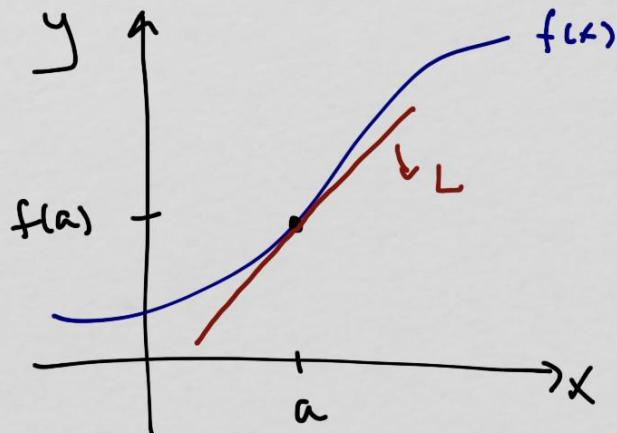
near  $x=a$ , the tangent line is approximately equal to the true curve  $f(x)$
