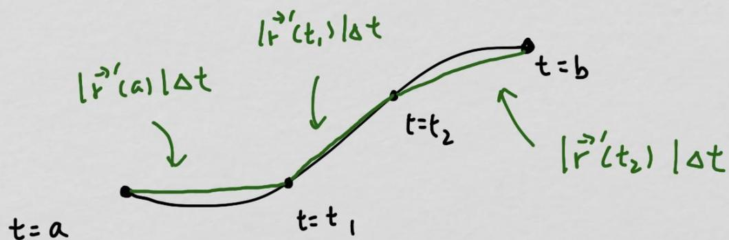
total length  $\approx |\vec{r}'(a)|\Delta t + |\vec{r}'(t_1)|\Delta t + |\vec{r}'(t_2)|\Delta t$
