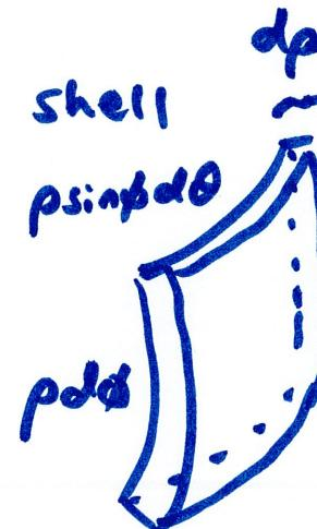
when  $dp$ ,  $d\theta$ ,  $d\phi$  are small, the shell is nearly a rectangular box
