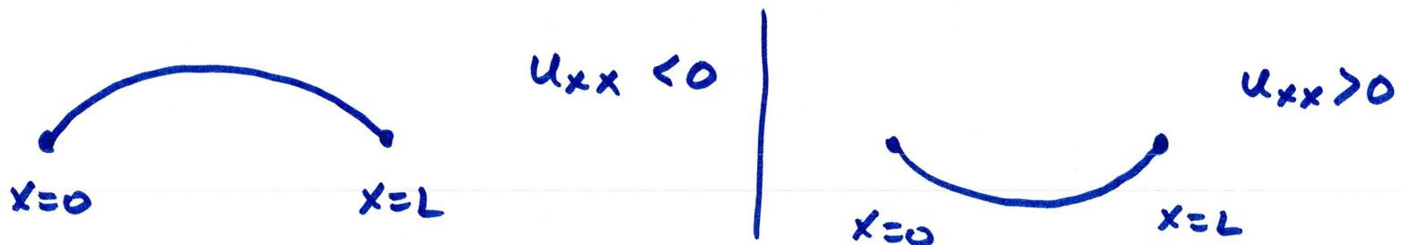
$u_{tt}$  is the acceleration (force) from the internal tension of string.  $u_{tt} > 0$  is upward force
