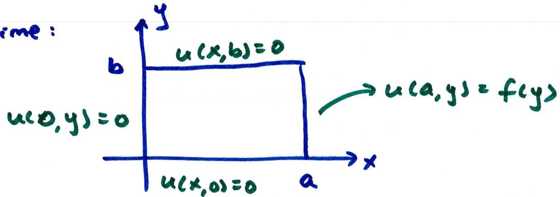
$$\text{Solution: } u(x, y) = \sum_{n=1}^{\infty} C_n \sinh\left(\frac{n\pi x}{b}\right) \sin\left(\frac{n\pi y}{b}\right)$$
