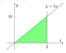
Notice that y ranges from the x-axis and the line y = 5x and x ranges from 0 to 2. Putting this in the double integral,
