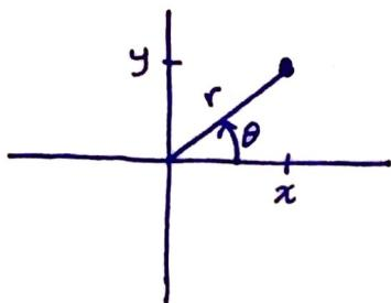
We can represent any point in Cartesian plane with an angle  $\theta$  and radius  $r$ . Positive angles are measured counterclockwise.
