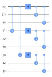
Figure 4: Quantum circuit for encoding.
