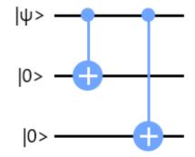
Figure 2: Quantum circuit for encoding.
