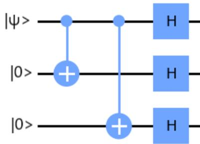
Figure 3: Quantum circuit for encoding.
