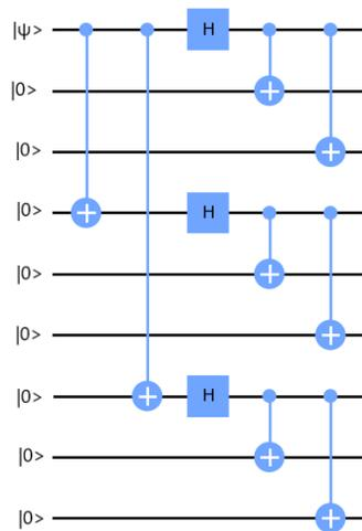
Figure 4: Quantum circuit for encoding.
