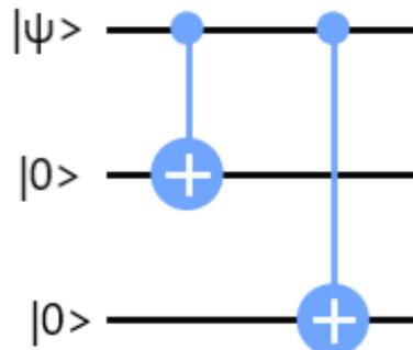
Figure 2: Quantum circuit for encoding.
