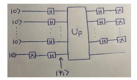
I claim that after measuring the output in the above circuit as indicated, we either see  $0 \cdots 0$  with probability 1 (in which case *F* is constant) or we do not see  $|0 \cdots 0\rangle$  with any probability (in which case *F* is balanced). Indeed, this follows from a fairly elementary calculation.
