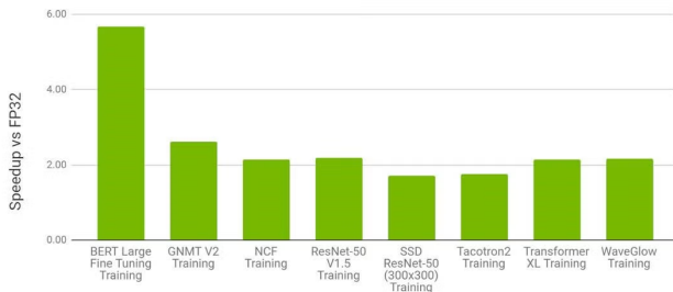
Figure: Performance of mixed precision training on NVIDIA 8xV100 vs. FP32 training on 8xV100 GPU. Source: M. Huang, C. Tekur, M. Carilli. Introducing native PyTorch automatic mixed precision for faster training on NVIDIA GPUs , PyTorch Blog (2020).
