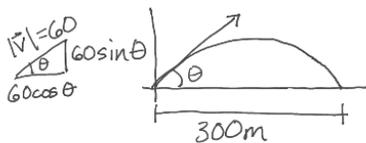
$$\begin{aligned}\vec{r}(0) &= \langle 0, 0 \rangle \\ \vec{v}(0) &= \langle 60 \cos \theta, 60 \sin \theta \rangle \\ \vec{a}(t) &= \langle 0, -9.8 \rangle\end{aligned}$$
