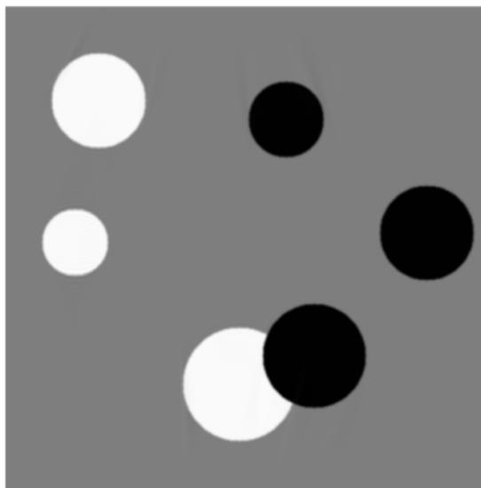
**Figure:** Full data Neumann series inversion, 10 terms,  $T = 5$ , on the square  $[-1, 1]^2$ , variable  $c = 1 + 0.3 \sin(\pi x^1) + 0.2 \cos(\pi x^2)$ . The artifacts are mainly due to the presence of corners. The  $L^2$  error on the left is 0.44%; and on the right: 0.34%. The  $L^\infty$  error on the left is about 1.2%; and about 3% on the right.
