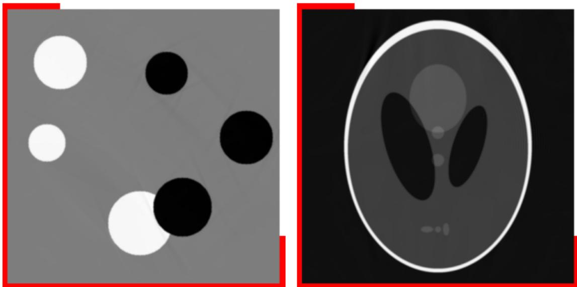
**Figure:** Partial data inversion with data on the indicated part of  $\partial\Omega$ . Neumann series inversion with 10 terms,  $T = 5$ ,  $\Omega = [-1, 1]^2$ . Left: constant speed  $c = 1$ ,  $L^2$  error = 0.7%. Right: **variable speed**  $c = 1 + 0.3 \sin(\pi x^1) + 0.2 \cos(\pi x^2)$ ,  $L^2$  error = 2%. Again, the most visible artifacts can be explained by the presence of corners.
