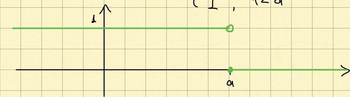
Plan: use  $u_a$ ,  $1 - u_a$  to model signals starting w/ time delay and/or stopping at a certain time.
