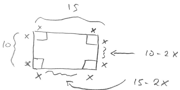
Objective function Volume, the variable  $x$  is the edge of the square being cut out
