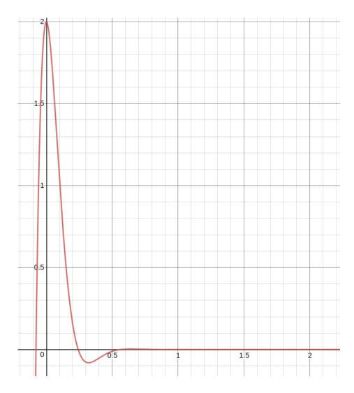
While not overdamped (there are still cosine and sine terms), the spring is very heavily damped, and the oscillations are not really visible on this graph.
