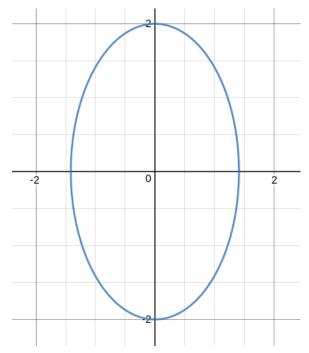
As t increases starting from 0, which corresponds to (u, u') = (0, 2), u, which is a sine function, starts to increase, and u', which is a cosine function, starts to decrease. So the point moves clockwise around the ellipse. (This is with u as the x-axis and u' as the y-axis; if you switch the axes, you get the opposite answer.)
