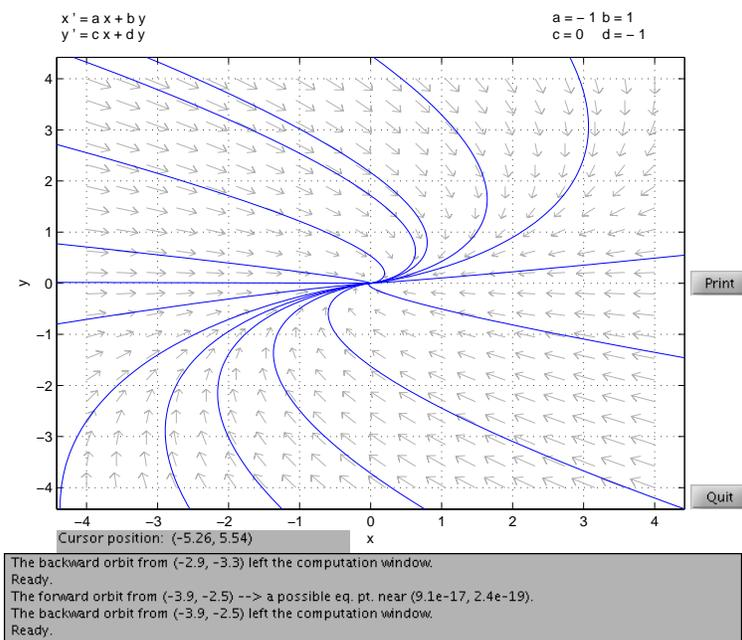
FIGURE 7. Improper stable node
