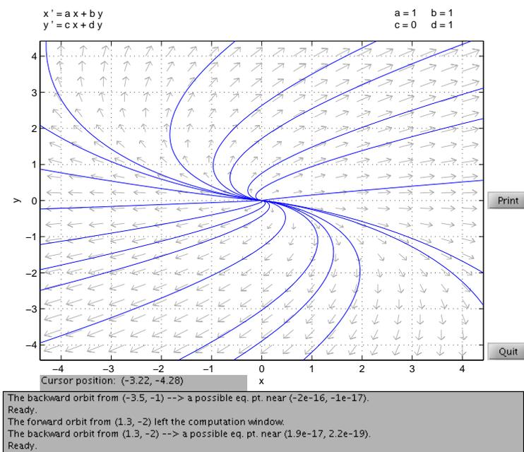
FIGURE 8. Improper unstable node
