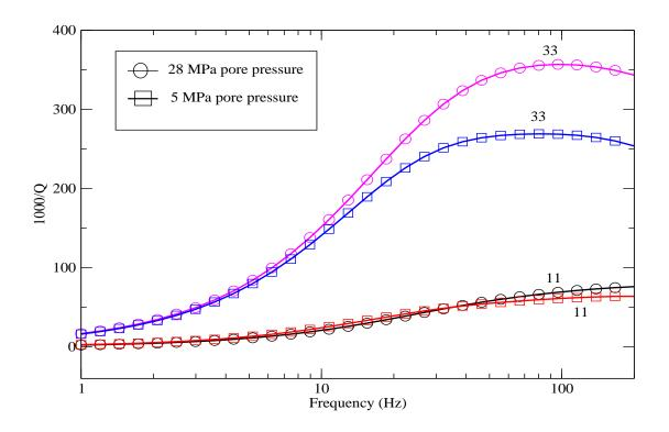
$\sigma=pc-pp$  is the effective normal stress, pc = confining pressure, pp= pore pressure. "11" and "33" refer to the qP wave along and perpendicular to the fracture plane. Attenuation is stronger in the overpressured case (circles) for "33" waves.
