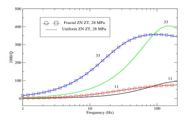
"11" and "33" refer to the qP wave along and perpendicular to the fracture plane. Dissipation factor of the "33" qP wave is more affected by the heterogeneities, showing lower values in the fractal case.
