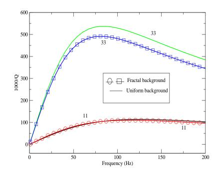
"11" and "33" refer to the qP wave along and perpendicular to the fracture plane. Phase velocities are lower for the fractal case for both "11" and "33" qP waves. Concerning attenuation, for qP "33" waves is lower than in the uniform background case, while attenuation for qP "11" waves is not affected by the fractal background.
