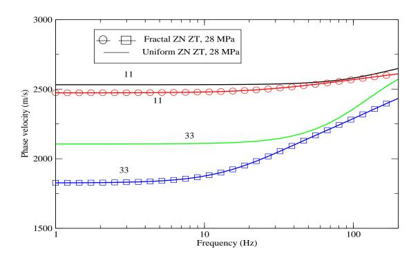
"11" and "33" refer to the qP wave along and perpendicular to the fracture plane. Phase velocities in the fractal case are lower than those obtained with the mean values. The "33" qP wave is the one more affected by the heterogeneities.
