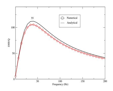
"11" and "33" refer to the qP wave along and perpendicular to the fracture plane. "55" and "66" refer to the qS and SH waves perpendicular and along the fracture plane. The SH wave is lossless. A very good fit is observed. qP waves along the fracture plane ("11") suffer lower attenuation than qP waves travelling perpendicular to the fractures ("33").
