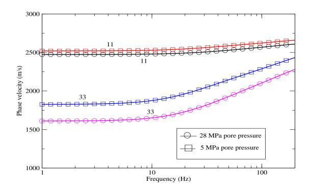
$\sigma=pc-pp$  is the effective normal stress, pc = confining pressure, pp= pore pressure. "11" and "33" refer to the qP wave along and perpendicular to the fracture plane. Higher pore pressure (circles) implies lower phase velocity. The "33" qP wave is the one more affected by overpressure.
