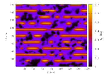
Fluid pressure distribution at 300 Hz in a brine-CO<sub>2</sub> patchy saturated sample with horizontal fractures. Numerical compressibility test for compression normal to the fracture plane.
