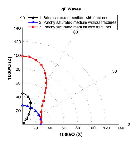
Fractures induce strong Q anisotropy for angles normal to the fracture plane, enhanced by patchy saturation.
