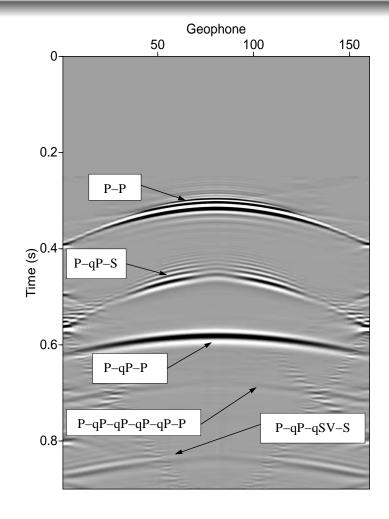
The seismograms show the arrivals of P and S waves reflected at the top of the HTI and VTI layers, as well as later arrivals corresponding to conversions from incident P to qP and qSV waves at the top and bottom of the layers. In particular, it is clearly seen the late P-qP-P arrival of the VTI case as compared with the corresponding one in the HTI case. The qP-velocities in the HTI and VTI layers are about 3800 m/s and 3000m/s, respectively.
