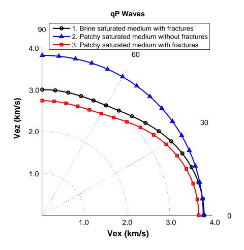
Velocity anisotropy caused by the fractures in cases 1 and 3 is enhanced for the case of patchy saturation, with lower velocities when patches are present. The velocity behaves isotropically in case 2.
