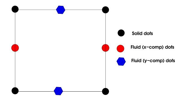
The solution of the oscillatory tests was computed using the FEM. The figure displays the local degrees of freedom (DOFs) associated with each component of the solid displacement and the fluid displacement vectors. Once we computed the  $p_{IJ}$  coefficients, we can determine the velocities and attenuation factors of the equivalent TIV medium.
