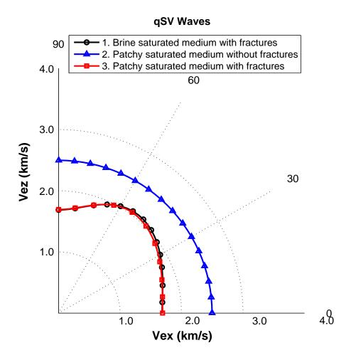
Velocity anisotropy is induced by fractures (cases 1 and 3). Patchy saturation does not affect the anisotropic behavior of the qSV velocities. Case 2 shows isotropic velocity, with higher velocity values than for the fractured cases.
