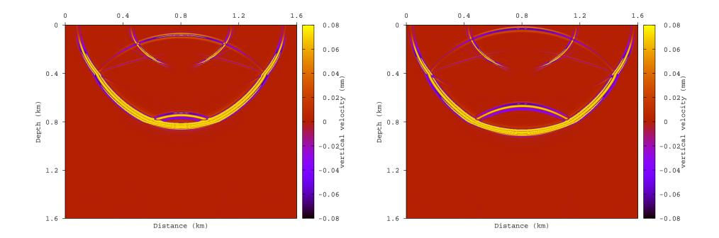
At 280 and 300 ms we can observe an upgoing P-wavefront and a tiny upgoing S-wavefront reflected at the top of the HTI layer and an upgoing qP-wavefront generated by reflection of the downgoing qP-wave at the bottom of the HTI layer. At 300 ms the reflected P-wave generated at the top of the HTI layer is arriving at the surface geophones.
