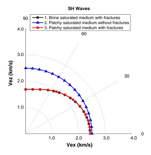
SH velocity anisotropy is observed to be induced by fractures. Cases 1 and 3 are almost indistinguishable.
