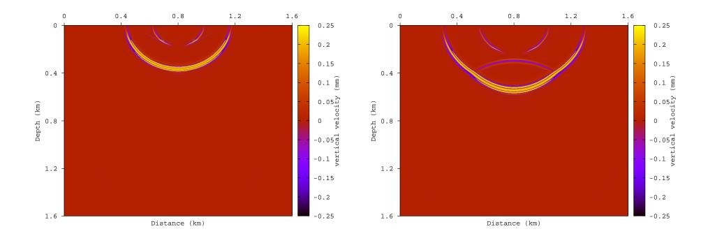
At 150 ms the incident P-wave is arriving to the top of the HTI layer. At 200 ms a reflected P-wave travelling upwards and a transmitted qP-wave travelling downwards are observed. The other wavefronts are S-waves generated by the point source at the top boundary.
