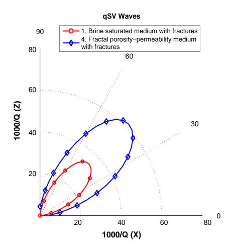
Note the increase in Q anisotropy for angles between 30 and 60 degrees
