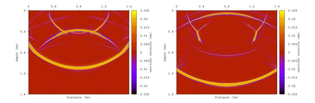
At 380 and 500 ms we can observe the reflected S-wave arriving at at the surface geophones, together with the qP-P wave reflected at the bottom of the HTI layer. The transmitted qP wave has already left the HTI layer and continues travelling downwards as a converted P-wave. Conversions to S-waves can also be seen in both snapshots
