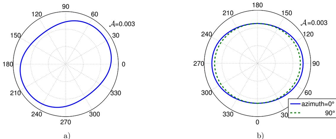
**Figure 13.** Horizontal (a) and vertical (b) cross-sections of the effective normalized attenuation coefficient for a model with relatively weak attenuation anisotropy. The model parameters are the same as those in Figure 11, except for  $\epsilon_Q^{(2)} = -0.1$ ,  $\delta_Q^{(2)} = 0.03$ , and  $\gamma_Q^{(2)} = -0.1$ .
