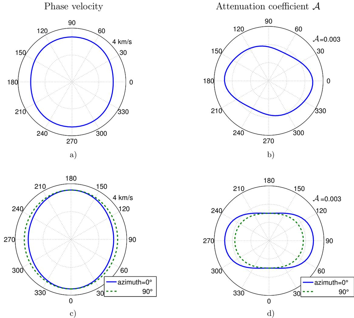
**Figure 12.** Effective P-wave phase velocity (left) and normalized attenuation coefficient (right) for the model from Figure 11. The velocity and attenuation are plotted in: (a,b) the horizontal plane as functions of the azimuthal phase angle; (c,d) the two vertical coordinate planes as functions of the polar phase angle.
