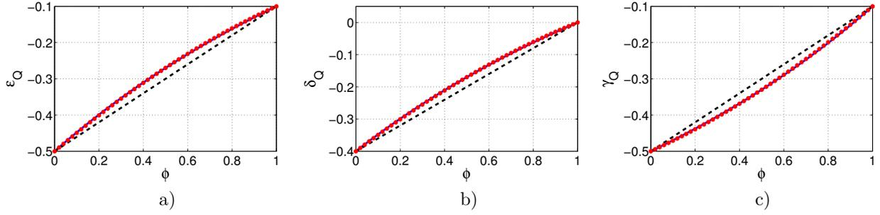
**Figure 4.** Effective attenuation anisotropy for a model with the same attenuation parameters as those in Figure 3, but both constituents have identical isotropic velocity functions ( $\epsilon^{(1)} = \epsilon^{(2)} = \delta^{(1)} = \delta^{(2)} = \gamma^{(1)} = \gamma^{(2)} = \Delta c_{33}/\bar{c}_{33} = \Delta c_{55}/\bar{c}_{55} = 0$ ). Compare with Figures 3d,e,f.
