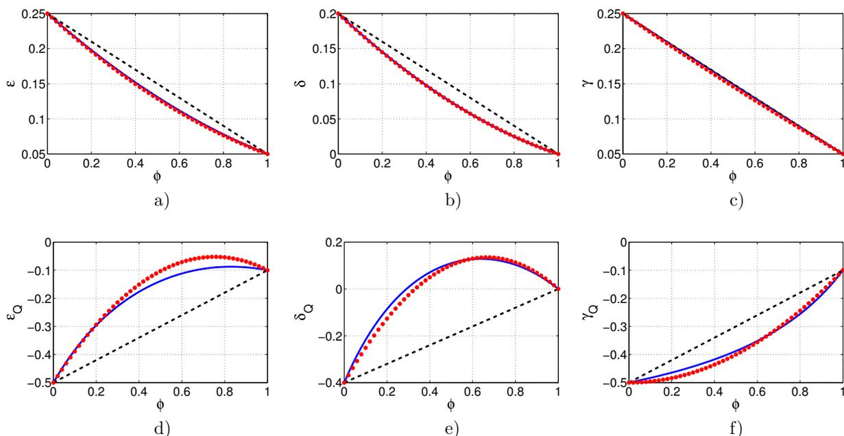
**Figure 3.** Effective velocity-anisotropy (a-c) and attenuation-anisotropy (d-f) parameters for the two-constituent VTI model from Table 1. The horizontal axis represents the volume fraction of the first constituent ( $\phi = \phi_1$ ). The exact parameters (solid lines) are plotted along with the first-order linear approximations (dashed) and the second-order approximations (dotted).
