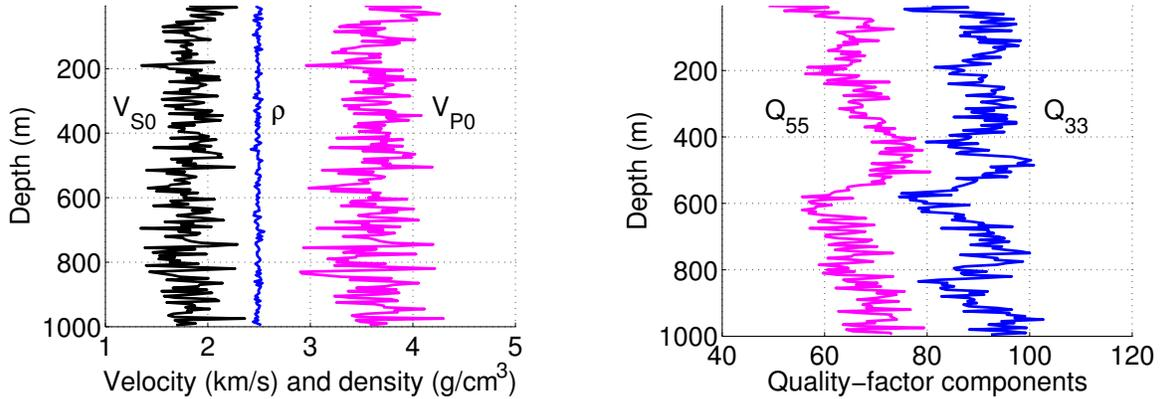
**Figure 7.** Vertical velocities, density, and the quality-factor components  $Q_{33}$  and  $Q_{55}$  of one realization of a model composed of VTI layers with VTI attenuation. The sampling interval is 5 m.
