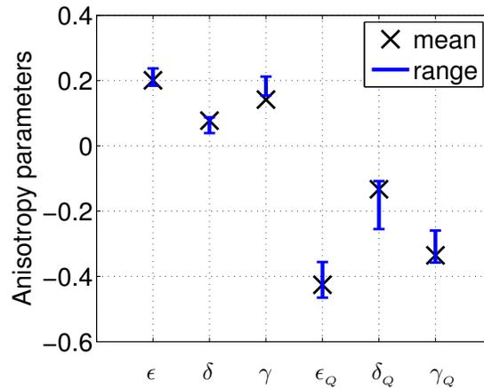
**Figure 8.** Mean values (crosses) of the interval anisotropy parameters and ranges (bars) of the exact effective parameters computed for 2000 realizations of the model from Figure 7. The standard deviations of all model parameters are listed in the text.
