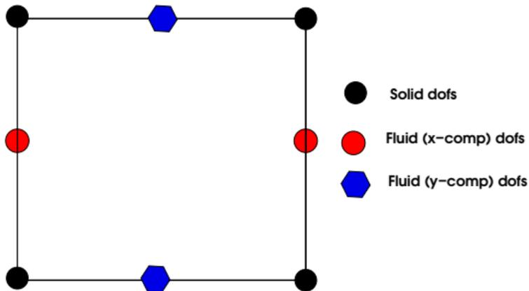
The solution of the oscillatory tests was computed using the **FEM**. The figure displays the local degrees of freedom (**DOFs**) associated with each component of the solid displacement and the fluid displacement vectors.
