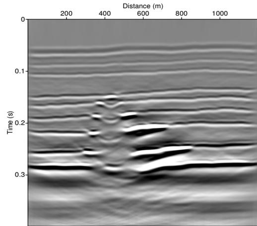
Figure 4: Synthetic seismogram after 1 year of CO<sub>2</sub> injection without updating the petrophysical properties.
