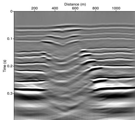
Figure 7: Synthetic seismogram after 2 years of CO<sub>2</sub> injection updating the petrophysical properties every 30 days
