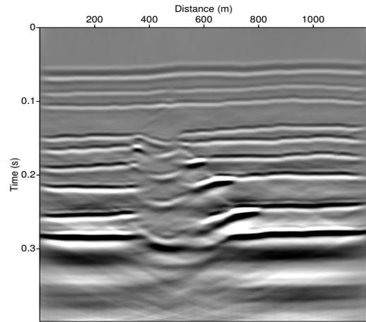
Figure 5: Synthetic seismogram after 1 year of CO<sub>2</sub> injection updating the petrophysical properties every 30 days
