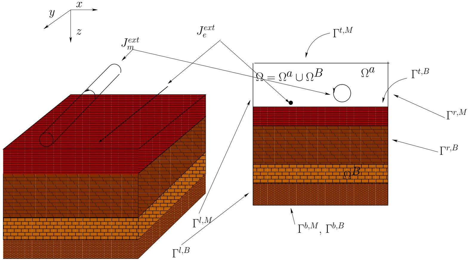
3D layered subsurface, 2D model  $\Omega = \Omega^a \cup \Omega^B$  and electromagnetic sources.
