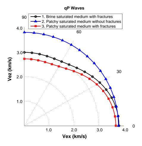
Velocity anisotropy caused by the fractures in cases 1 and 3 is enhanced for the case of patchy saturation, with lower velocities when patches are present. The velocity behaves isotropically in case 2.
