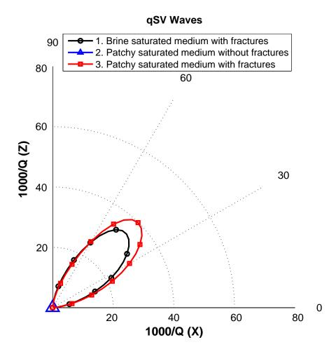
qSV anisotropy is strong for angles between 30 and 60 degrees. The lossless case 2 is represented by a triangle at the origin.
