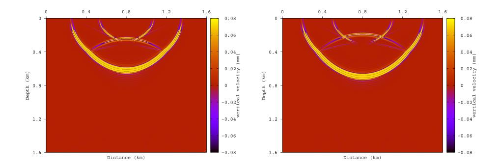
At 220 ms and 240 ms a reflected P-wave and travelling upwards and a transmitted qP-wave travelling downwards are observed. Note the deformation of the qP-wavefront because of the anisotropy in the HTI layer.
