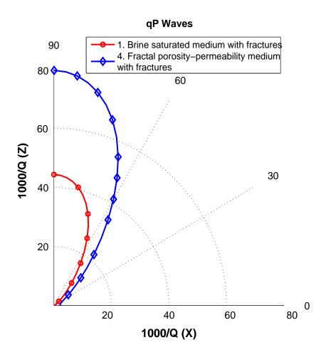
Note the increase in Q anisotropy for qP waves for angles normal to the fracture plane.
