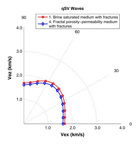
Note the (small) increase in Q anisotropy for qSV waves for angles between 30 and 60 degrees.
