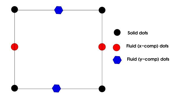
The solution of the oscillatory tests was computed using the FEM. The figure displays the local degrees of freedom (DOFs) associated with each component of the solid displacement and the fluid displacement vectors. The apriori error estimate in the energy norm is on the order of  $h^{1/2}$ . Once we computed the  $p_{IJ}$  coefficients, we can determine the velocities and attenuation factors of the equivalent TIV medium.
