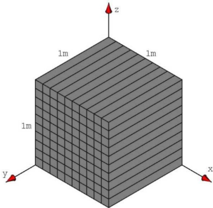
Fluid-saturated fractured poroelastic sample.
