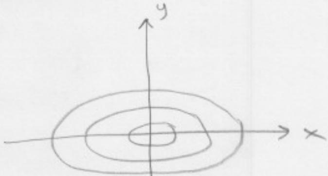
The level curve of  $f$  at  $c$  is the projection on to the plane  $x-y$  of the intersection of the graph of  $f$  with the plane  $z=c$ .
