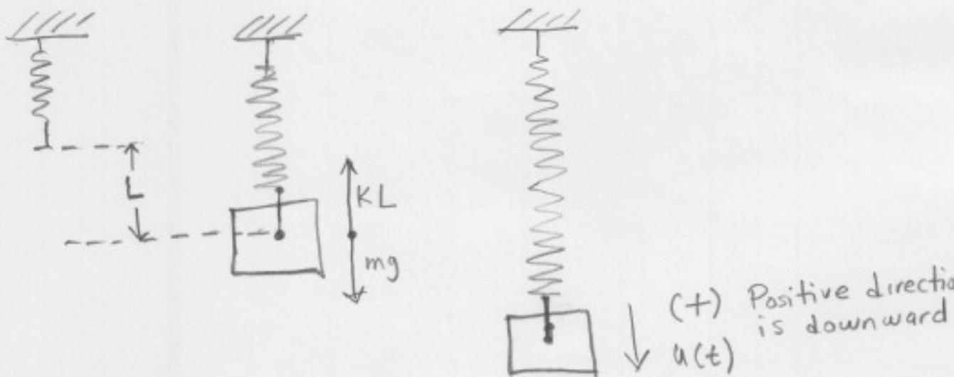
A mass  $m$  hangs from vertical spring. The mass causes an elongation  $L$  of the spring.
